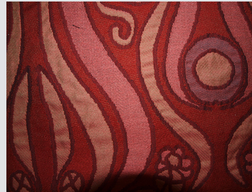
In 2014, RISD offered a Jacquard class with Convergence. This is a doubleweave design - fine cotton warp and rayon weft.
