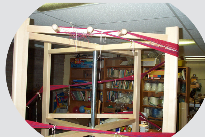
Large warping mill for making weaving warps
