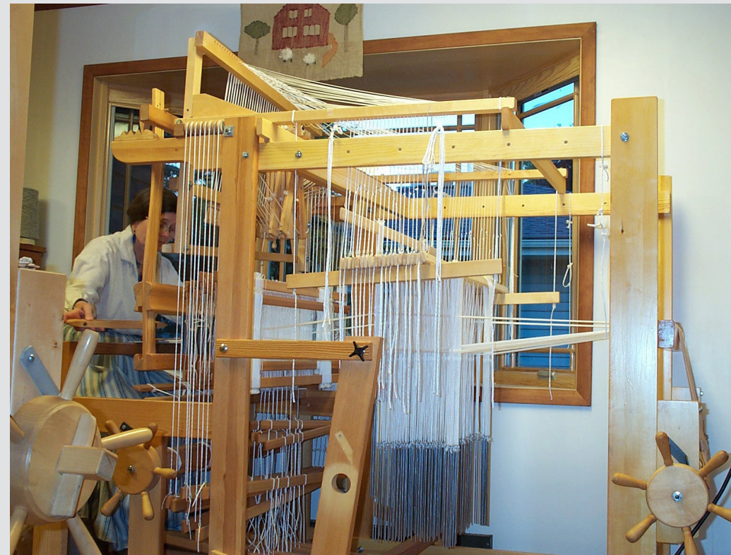
Lilla 100cm loom with Myrehed 50 pattern shaft draw system for damask
